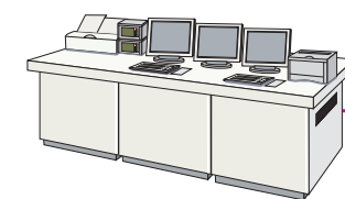
General-purpose building control computer (LONWORKS® device)
